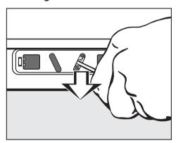
■ Insert a screwdriver into the notch of the right opening and pull downwards. The door will now open.
